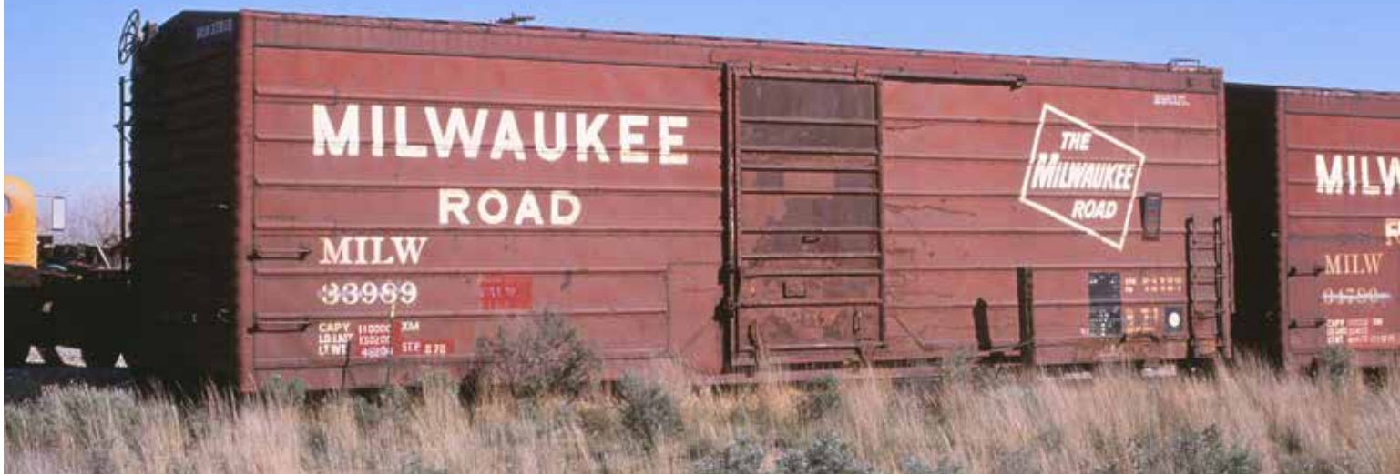
ABOVE MILW 33989 was a 40-foot 2SD rib-side XM boxcar, photographed at Othello, Wash., on April 11, 1988. BOB BOELTER COLLECTION
