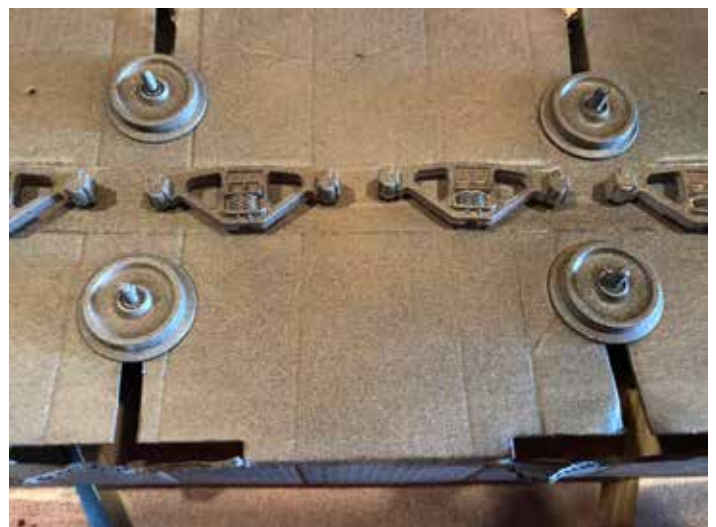
ABOVE Bob's chopped up cardboard box allowing wheels to be slipped in for painting.
