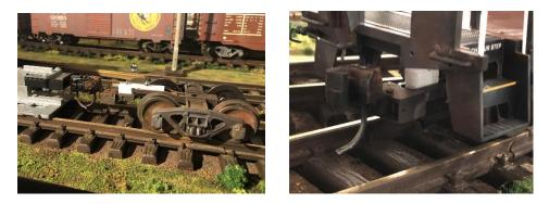
So, a bridge between the couplers and the bar from the truck had to be created. Here (in white) it is being tested to a Kadee height gauge. Prototype photos show the bar from the underframe is heavy-duty steel and muscular. Here the solution looks anemic.
