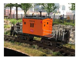
The finished model with light weathering and decals applied. The roof has a smoke stack (USAT), a small vent, roof walks (USAT) and distinctive roof railings. There's one problem. The truck-mounted couplers are hidden because of the length of the porches.
