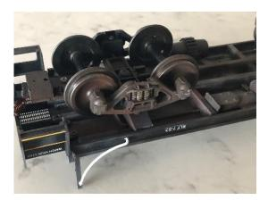
Here is a close-up of the painted and weathered underframe. In the previous picture you'll notice I chose Kadee 831 truck-mounted couplers with a large offset. I did this not wanting to mount a coupler box directly to the see-through tread between the stairs. The tradeoff is that USAT trucks have a low mounting bar to suit their proprietary couplers.
