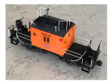
The final result with extended couplers. The end castings, with brake wheels, are what USAT calls "Bay window caboose ladder assembly". I moved the ladders to the caboose body.
