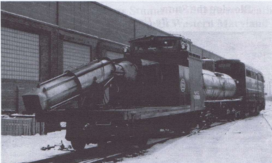
One of the early New York Central Jet snow blowers. New York Central photo from the Don Wetzel collection
