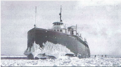
One of the PM car ferries is shown surrounded by ice. This appears to be the sheet ice that the boats could break up either by cutting through it or by riding up on it.
