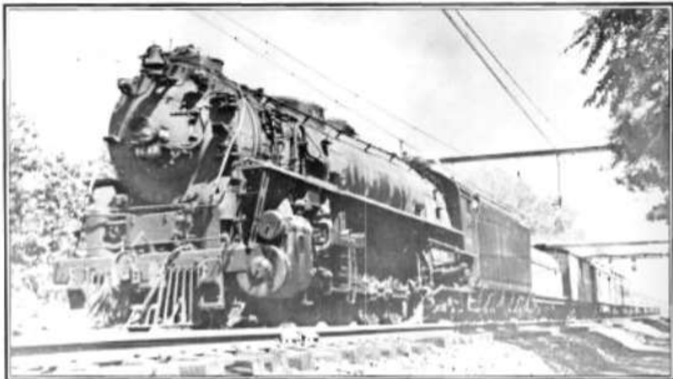
EASTBOUND LACKAWANNA PASSENGER TRAIN at East Orange, New Jersey, on May 26, 1936. The first two cars behind DL&W 4-8-4 No. 1643 were "BFIX" Borden bulk-milk tankcars.
